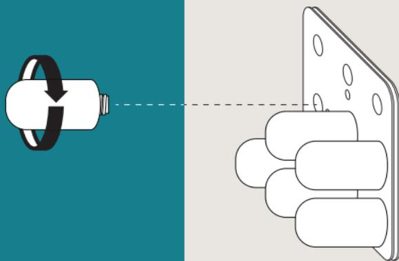
As an alternative, the baseplate can be mount with adhesive tape
